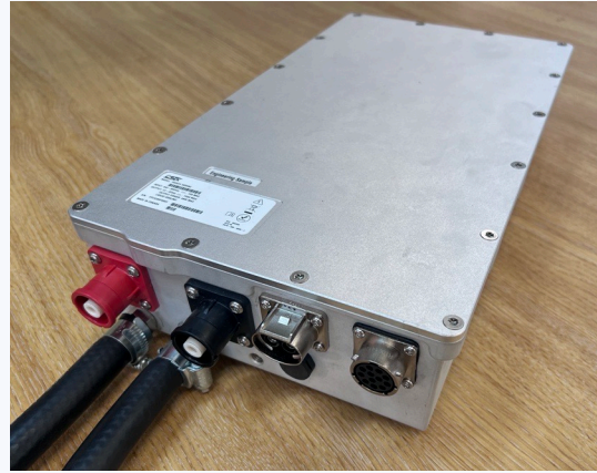
Lyra's 4kW SiC DC-DC Converter
