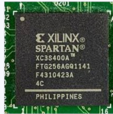
An FPGA chip on the PCB
