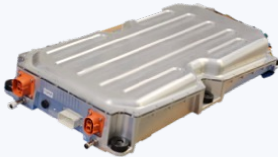
Lyra's 22kW SiC Bi-directional On-board Charger
