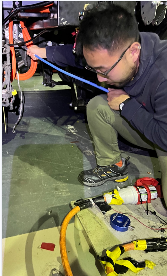
Measuring surface currents on the vehicle chassis
