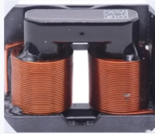
Flat-wire winding on a sectional wound CMC
