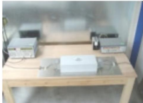
Figure 3 Test set-up for filter insertion loss
