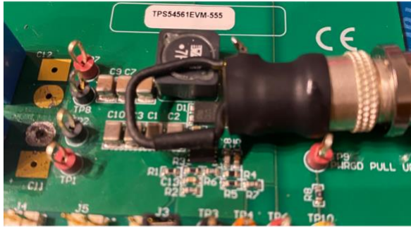
(a) a magnetic field loop is placed over the “hot loop” area
