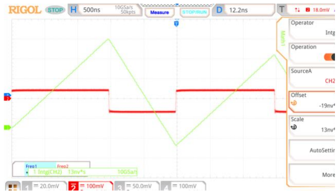
Figure 9 Placing the loop over the inductor gives the induced voltage caused by current going through the inductor. The integration of the waveform gives the inductor current waveform
