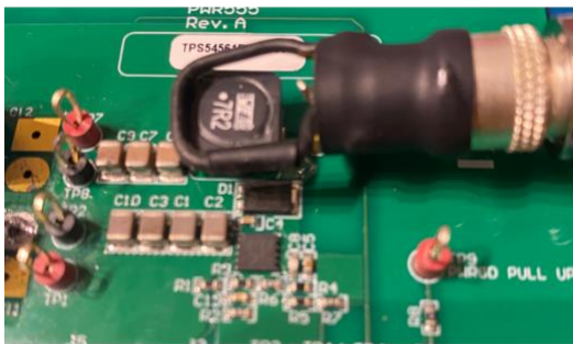
Figure 9 Placing the loop over the inductor gives the induced voltage caused by current going through the inductor. The integration of the waveform gives the inductor current waveform
